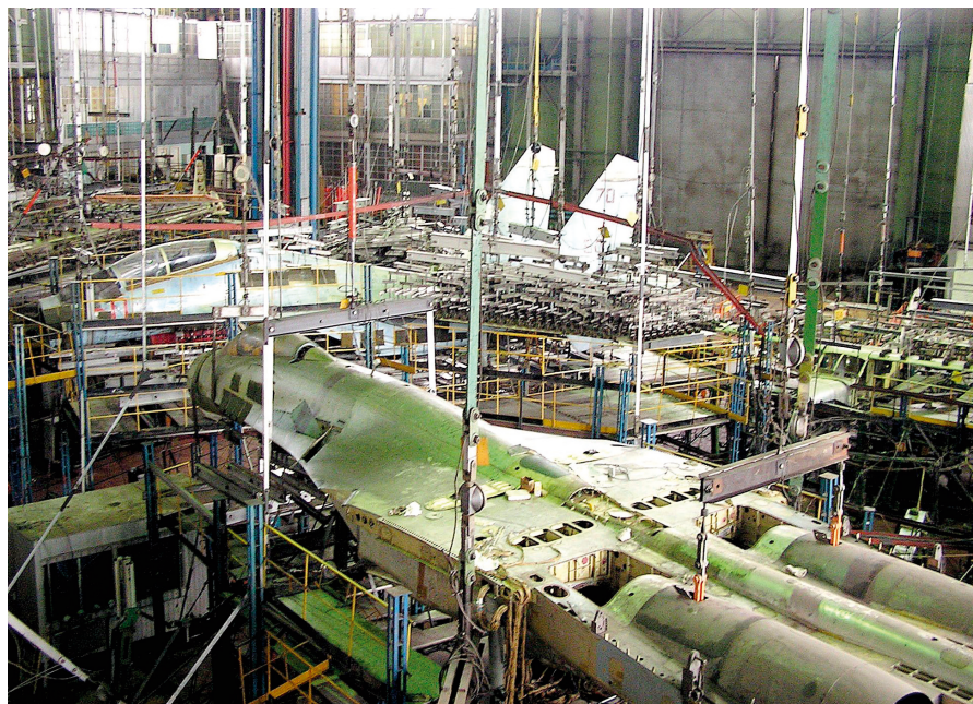
Full-scale samples in the endurance and static testing hall
