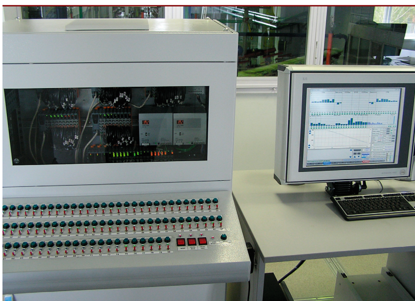
SUPERJET endurance test stand control station
